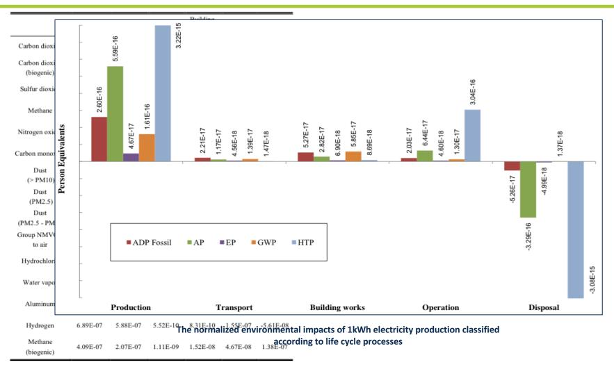
Emissions to air per kWh electricity production
